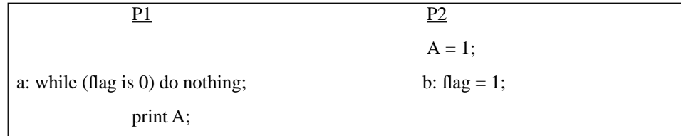
Figure 2-14 Point-to-point event synchronization using flags.
